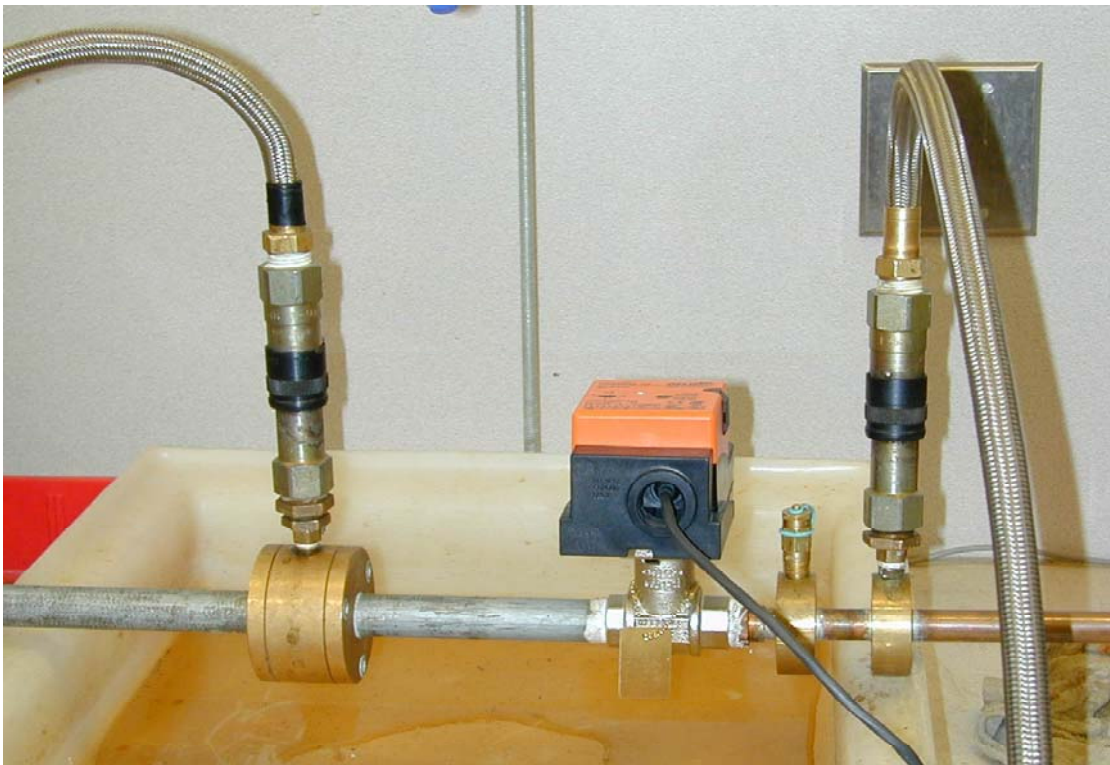
Plate 2 1/2 inch CCV valve under test. Flow from right to left
