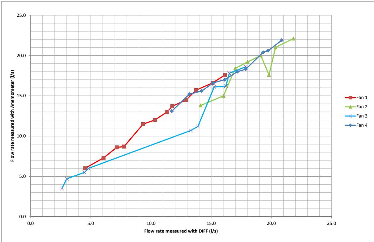
Figure 3 TSI Anemometer vs DIFF Results
