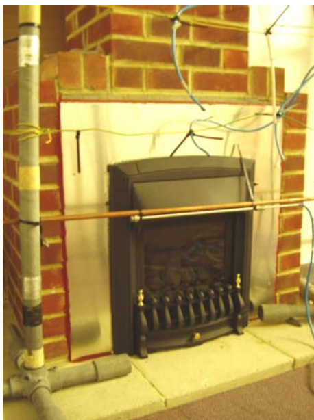
Figure 5 ILFE Fire showing position of sampling sparge bar
