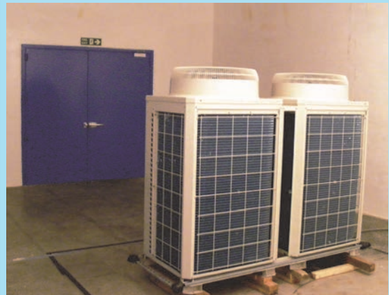
Mitsubishi Electric Ecodan unit under test in BSRIA's new acoustic chamber
